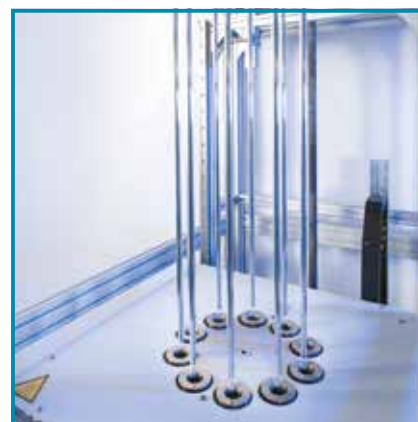
Burette tubings are manufactured by using vacuum technology to maintain diameter of the burette tubings uniform all over their length.
