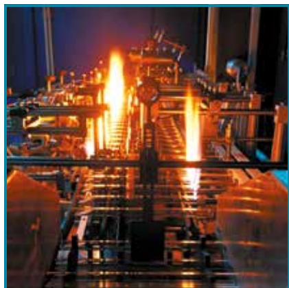
All joints are manufactured by automatic forming machines for consistent quality and guaranteed uniformity.
