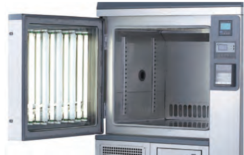
Built-in cool white fluorescent lamp and UVA lamp
